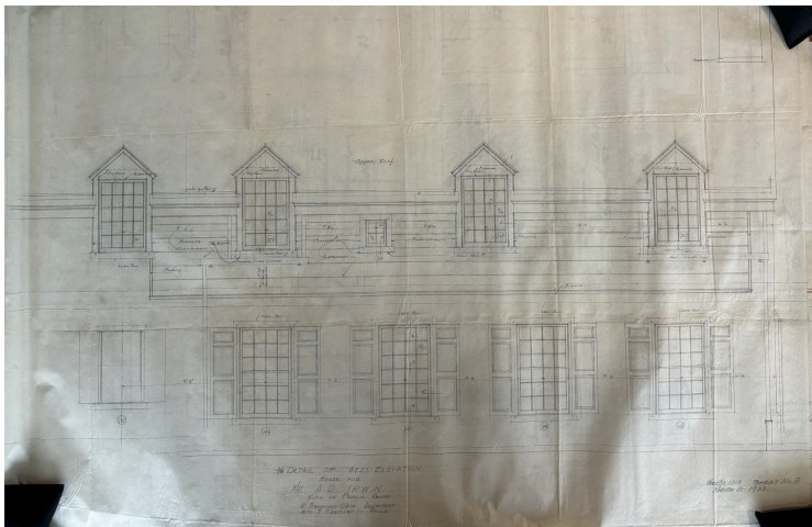
Fig. 5. West side elevation drawing of the 1932 addition showing partial clapboard siding. From the R. Brognard Okie Architectural Papers. Photographed at the Pennsylvania State Archives in Harrisburg.
