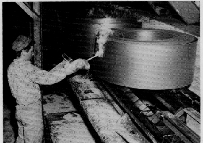
Coils are marked with order number, while still hot, after coming from the Hot Strip coiler.
