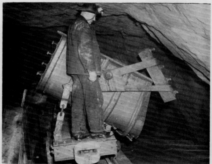
A gramby self-dumping ore car, which carries the ore from the chute to the ore pocket, and drops into the crusher and broken into chunks for hoisting to the surface.
